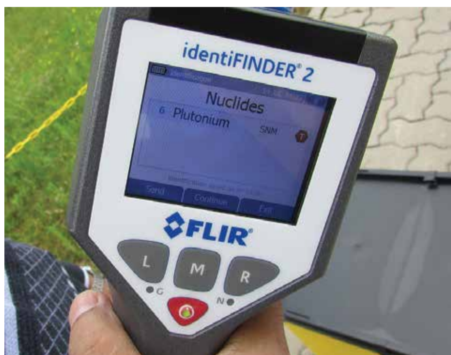
PICTURE 2: Portable measuring instrument for the identification of radiation sources (Source: EUSECTRA)
